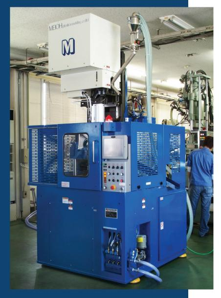
In order to manufacture an high precise insert molding product, a high precise molds and dies are required, of course an automatic insertion system, kinds of automatic checking systems and automatic packing system, etc. are required too.
